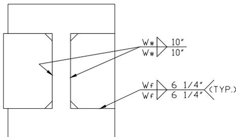
(a) stiffeners welded to column
