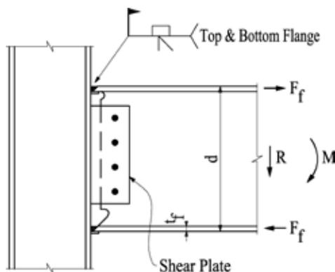
▲ Fig. 1: Directly welded moment connection.
