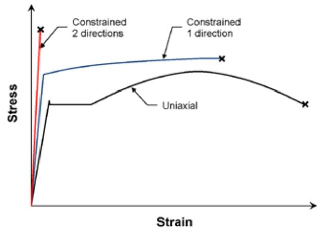
▲ Fig 4. Stress-strain curves for steel under various levels of restraint.
