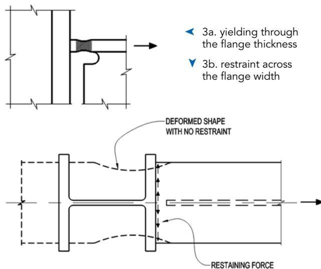
Fig. 3. Restraint at the beam flange.
